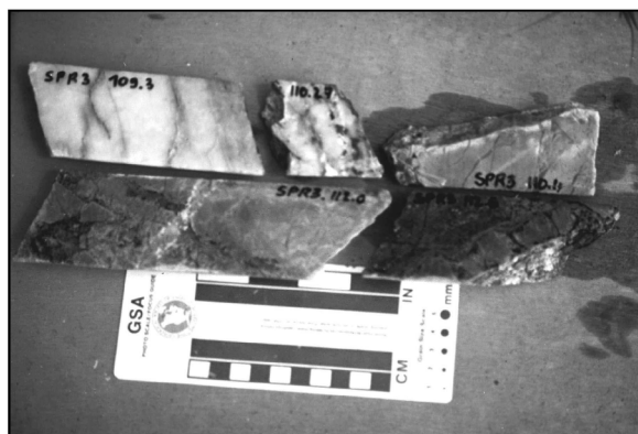
b. Drillhole samples from Saint-Pierre showing the contact between the gold-bearing quartz vein and the albitized granite sill
