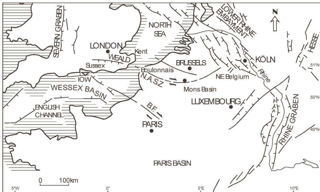
Fig. 1.- Tectonic framework of NW Europe (Belgium, north of France and U.K.) with the main crustal structures active in terms of brittle structures during the Meso-Cenozoic. NASZ : North Artois Shear Zone, B.F.: Bray Fault. The Cretaceous formations have been investigated in particular in the Isle of Wight (IOW), Sussex, Kent, Boulonnais, Mons Basin and NE of Belgium.
